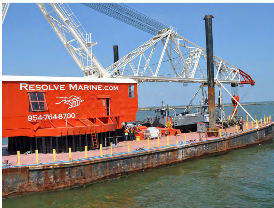
Figure 1-3. Resolve spud barge with 2 MARCO Class V skimmers on deck departing Gulfport. Barges provided secure storage for the skimmers and their crew when weather conditions exceeded their seakeeping capability.
