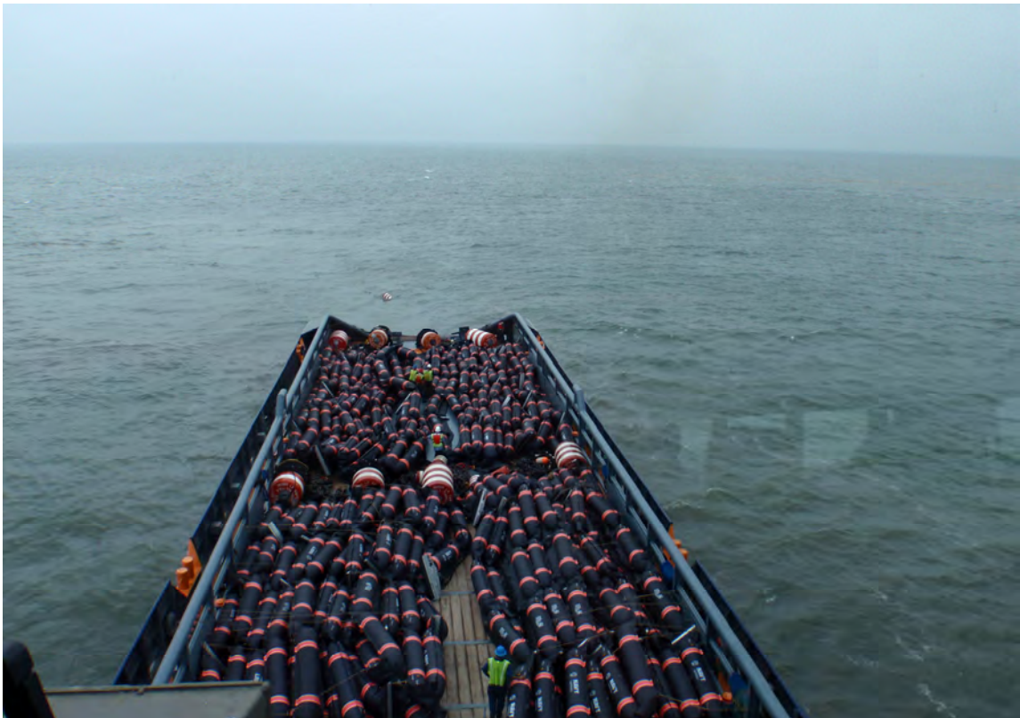
Figure 3. 4000' of Oil Containment Boom with Boom Mooring Systems On Board the OSV MV John Coghill
