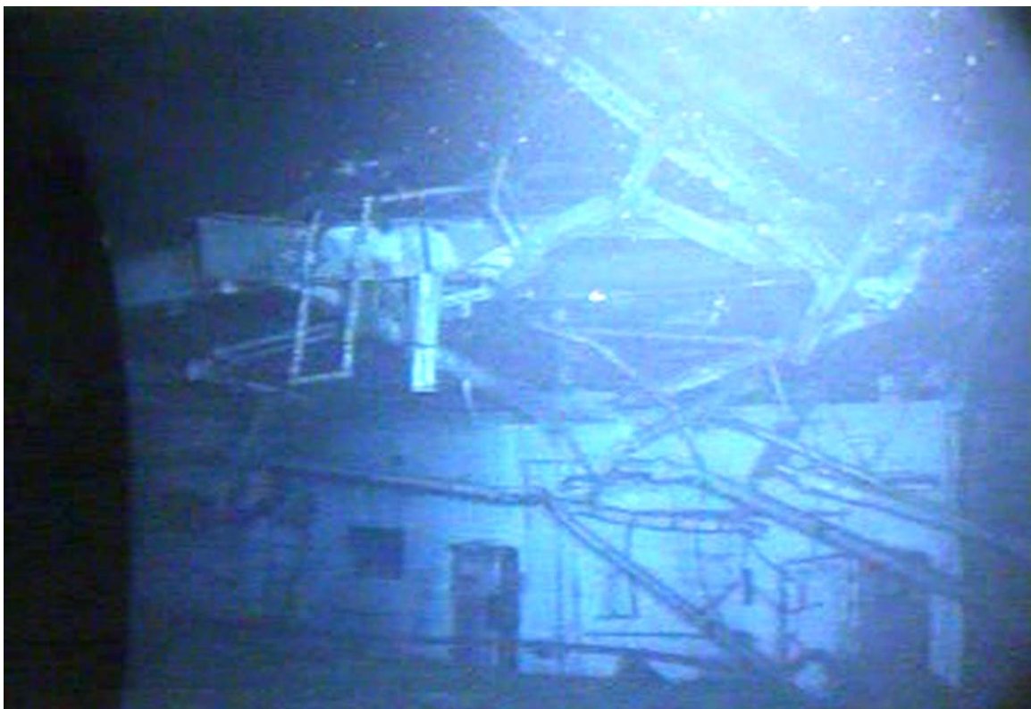
Photograph 14: Bridge Control Room with Helicopter Deck Wreckage
