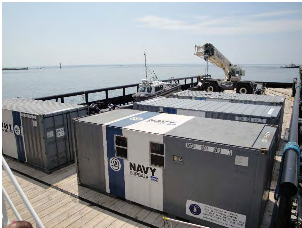
Figure 5-8. Stern deck of OSV BAYOU BEE configured with crane and shop vans to provide mobile MARCO Class V skimmer maintenance.
