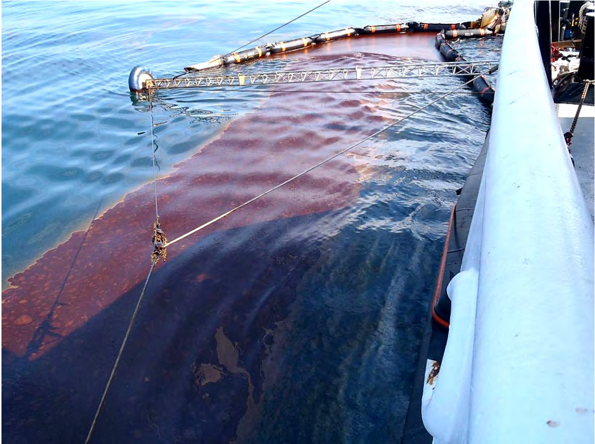
Figure 17. Skimming Using the Outrigger Assembly and Class XI Skimmer System
