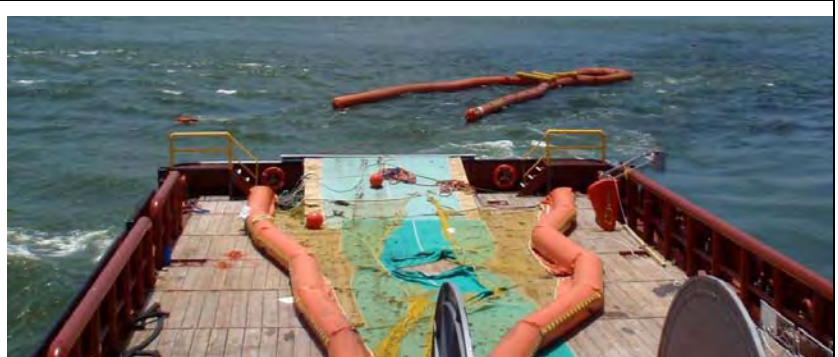
Figure 3: View towards stern of an OSV crabbing forward (12 degrees) to use the side of the vessel to help direct oil into skimmer and pocket.
