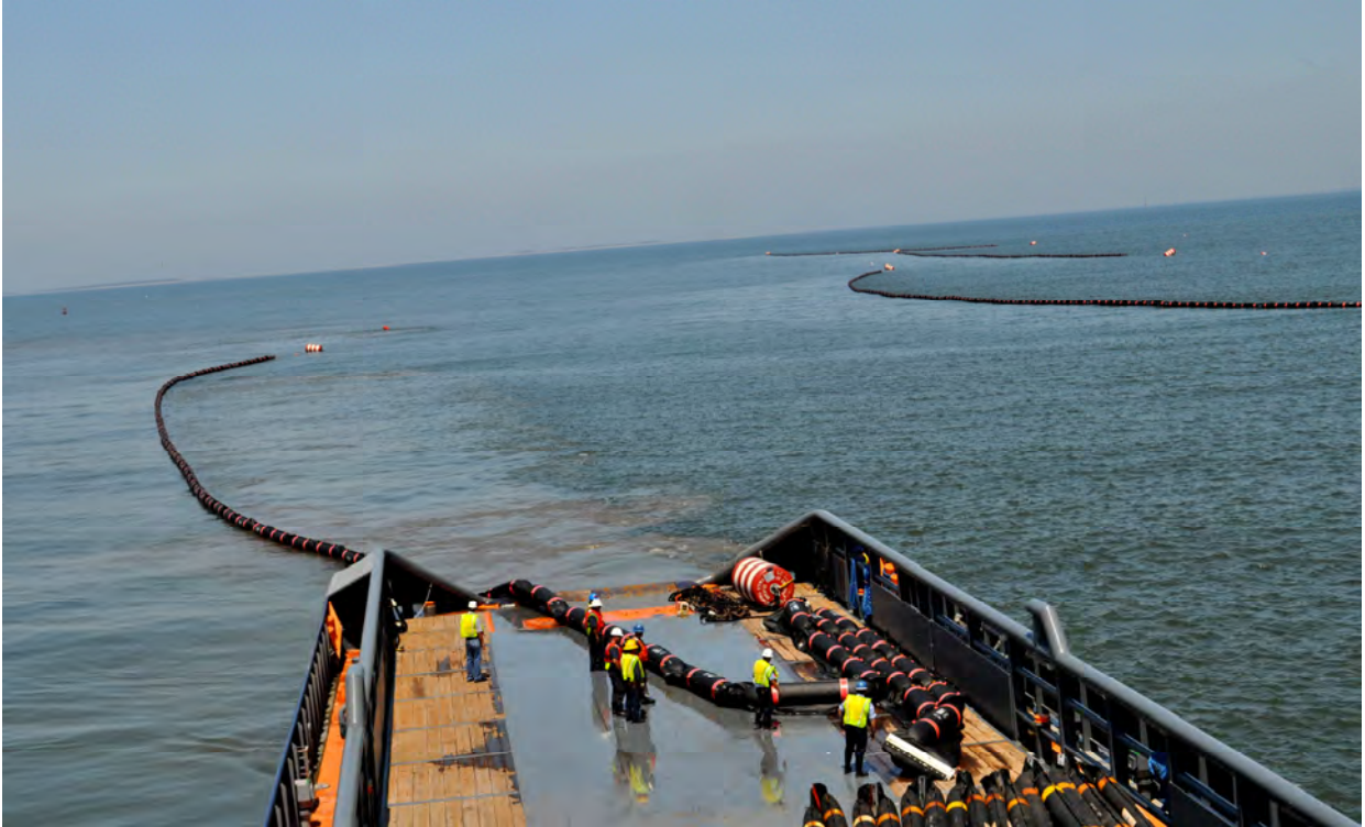
Figure 6. Oil Containment Boom Deployed off the Western Tip of Ship Island in a Cascade Configuration
