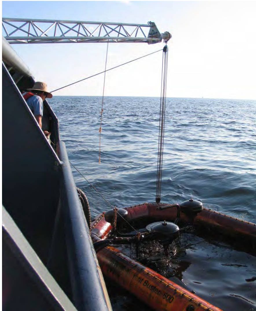
Figure 5-13. Outrigger Assembly suspended over the side rail used to service the pump in the pocket of the High Speed Current Buster
