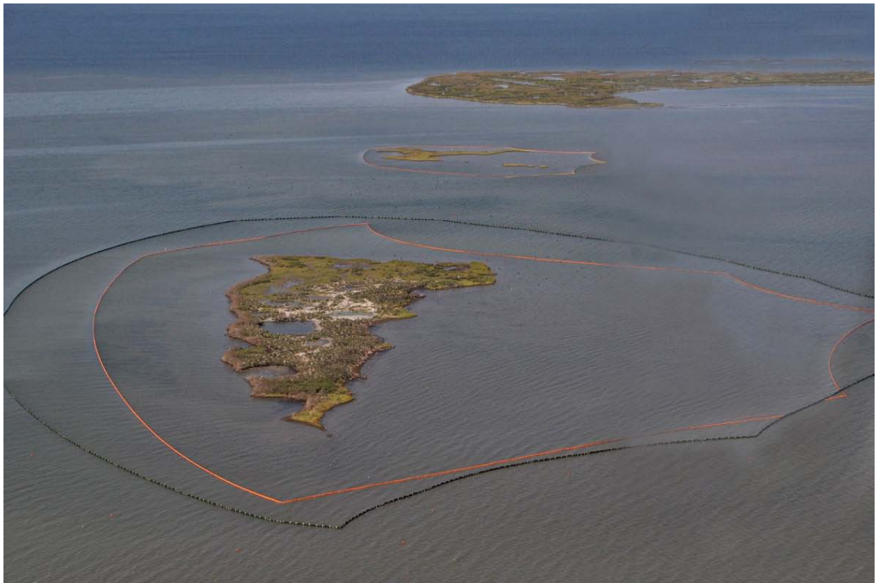
Figure 6-3. 26" SUPSALV boom completely circling New Harbor Island, part of the Chandeleur Islands east of New Orleans.
