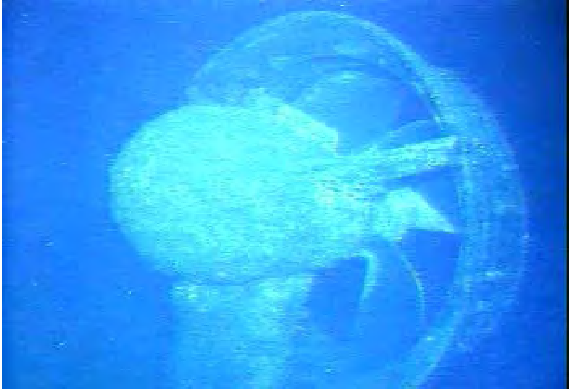
Photograph 9: Deep Water Horizon Megastar Thruster Pod
