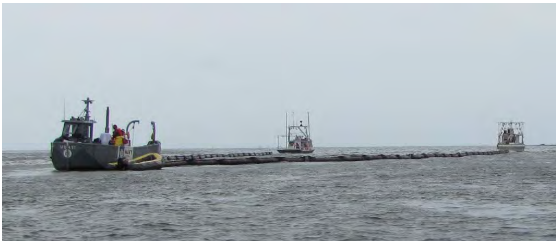
Figure 5-6. MARCO Class V being towed by its booms by two gulf shrimpers.
