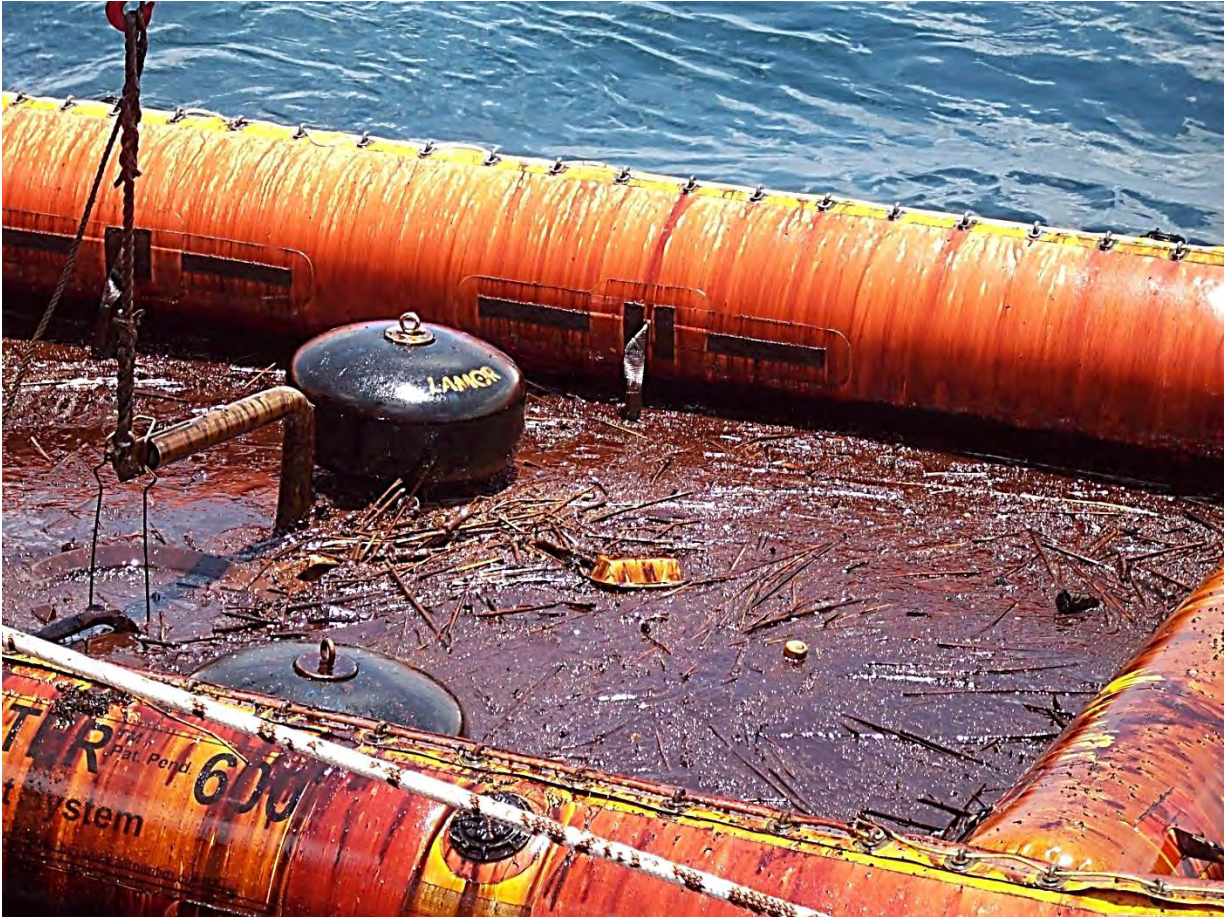
Figure 13. Oil and Debris Mix in Pocket of High Speed Current Buster VOSS
