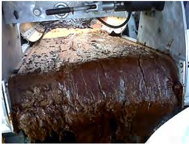
Figure 16. Crude Oil Rolling off Skimmer Belt
