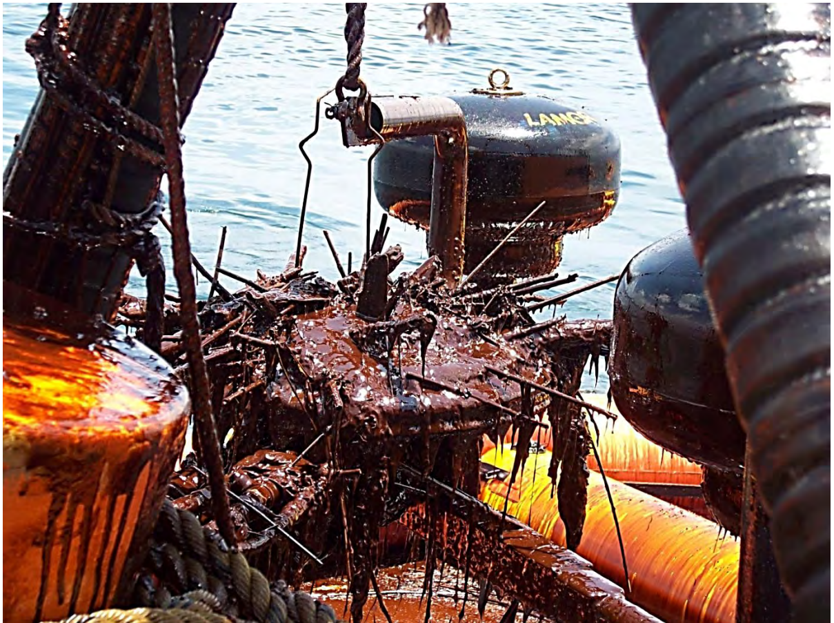
Figure 14. Oil and Debris Mix on Weir Skimmer in High Speed Current Buster VOSS
