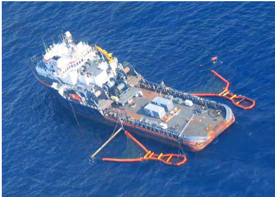
Figure 5-10. OSV VANGUARD pulling two NOFI High Speed Current Busters on the afternoon of 28 May, 2010. The port side NOFI is deployed with an outrigger assembly and the starboard side NOFI is employing a paravane to hold the boom open.
