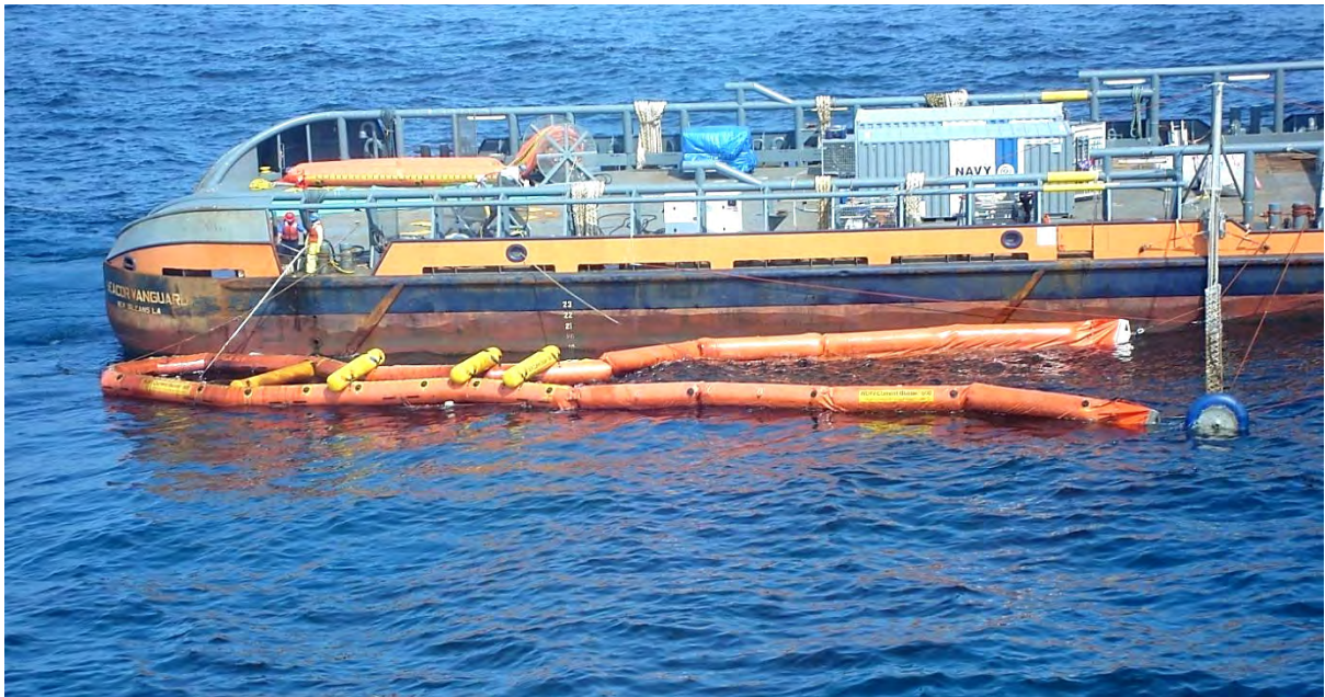
Figure 12. OSV AHTS Vanguard Recovering Spilled Oil Using High Speed Current Buster
