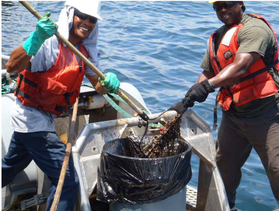
Figure 5-12. SUPSALV crew maintaining the proper attitude while cleaning debris from the belt of the Class XI skimmer while deployed on OSV RENE (11 June 2010)
