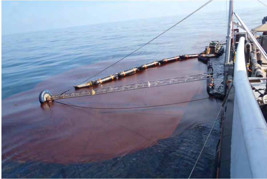
Figure 5-9. VOSS Class XI Sorbent Belt Oil Skimmer deployed on OSV RENE pulling through a thick pocket of oil.
