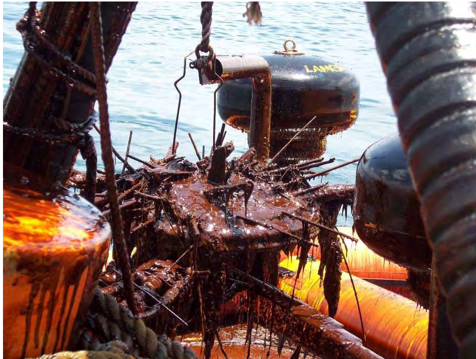
Figure 5-11. OSV JOHN COGHILL's High Speed Current Buster weir pulled from water to allow cleaning of debris which was clogging suction.
